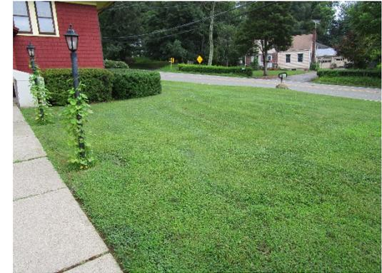
Two identical bioretention systems can be installed on either side of the dividing sidewalk to infiltrate the water from the downspouts on either corner of the front side of the library. Another rain garden can be installed to capture, treat, and infiltrate stormwater runoff from the parking lot. A preliminary soil assessment suggests that the soils have suitable drainage characteristics for green infrastructure.
