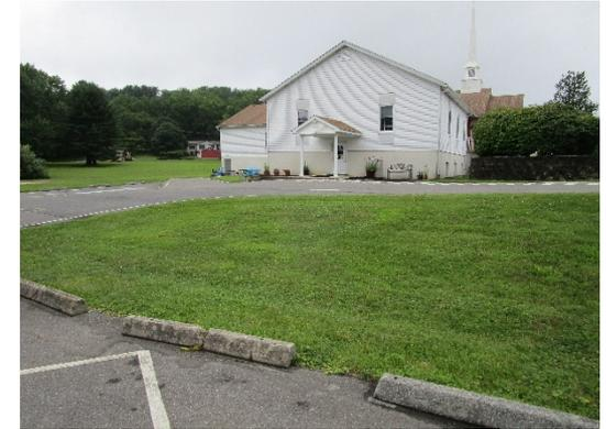
Pervious pavement can be installed in the northern section parking spaces to capture and infiltrate the runoff from the parking lot. A rain garden can be installed in the center island to capture, treat, and infiltrate stormwater runoff from the driveway. Planter boxes can be installed on the building to treat the rooftop drainage area. A preliminary soil assessment suggests that the soils have suitable drainage characteristics for green infrastructure.
