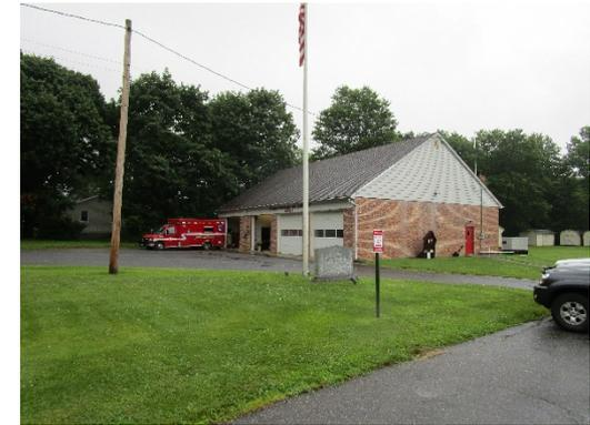
Two cisterns are proposed on the front of the firehouse to recycle rainwater. In addition, a bioretention system can be installed to treat the runoff from the parking lot. A preliminary soil assessment suggests that more soil testing would be required before determining the soil's suitability for green infrastructure.
